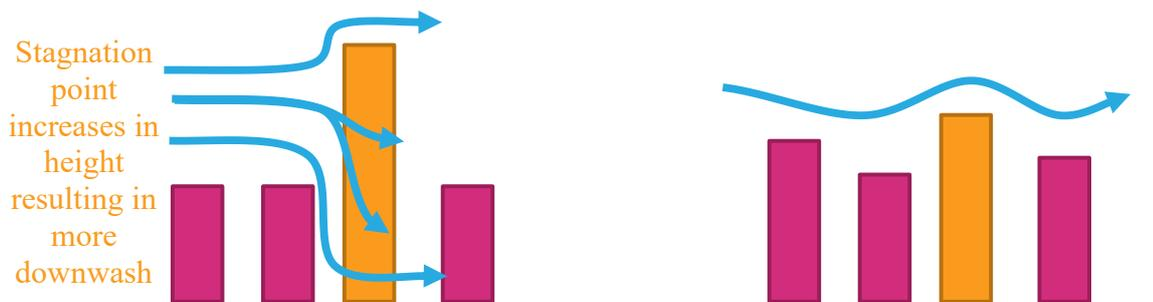
Figure 30 Schematic of flow pattern interference from surrounding buildings
