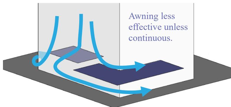
Figure 27 Schematic flow pattern around building with awning
