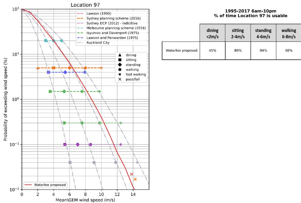
Figure 15: Probabilistic comparison between wind criteria based on mean wind speed (for the hours of 6 am and 10 pm) – Location 97
