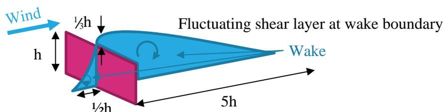
Figure 32: Sketch of the flow pattern over an isolated structure
