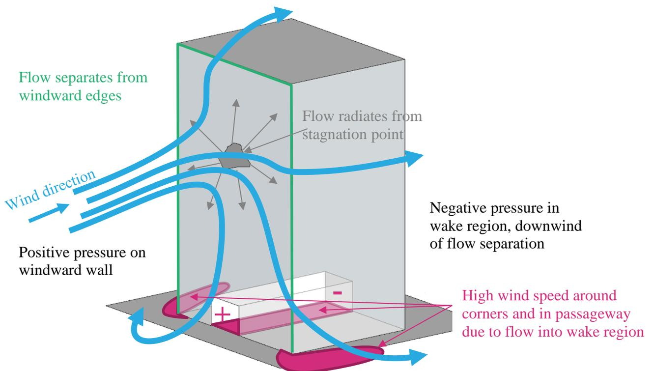
Figure 25 Schematic wind flow around tall isolated building
