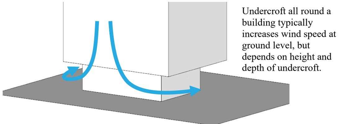
Figure 28 Schematic of flow patterns around isolated building with undercroft
