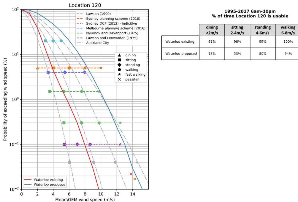
Figure 6: Probabilistic comparison between wind criteria based on mean wind speed (for the hours of 6 am and 10 pm) – Location 120
