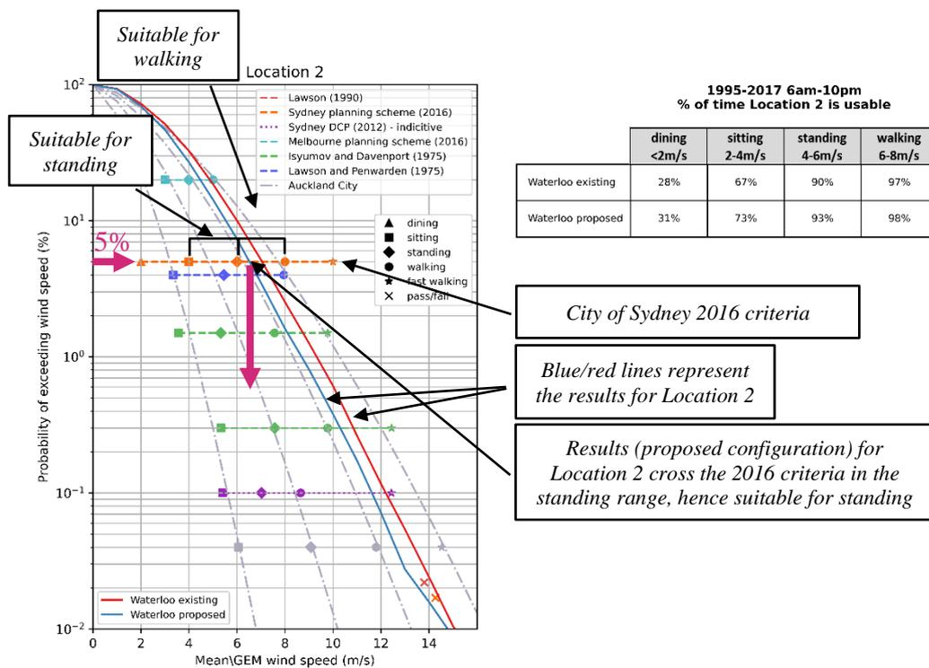
Figure 5: Probabilistic comparison between wind criteria based on mean wind speed (for the hours of 6 am and 10 pm) – Location 2
