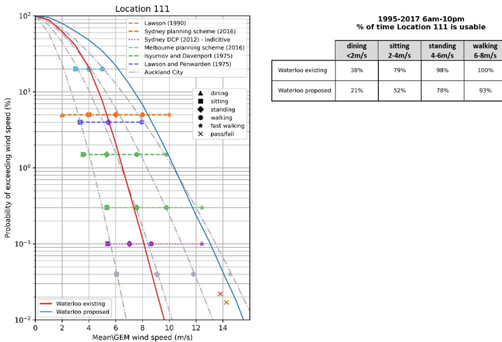
Figure 9: Probabilistic comparison between wind criteria based on mean wind speed (for the hours of 6 am and 10 pm) – Location 111
