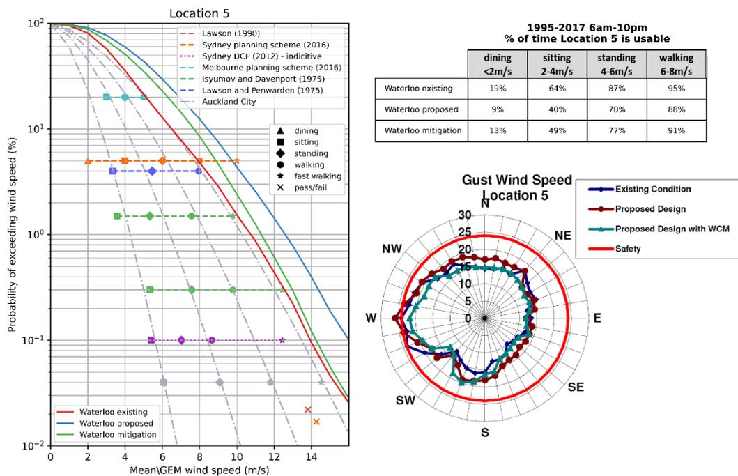
Figure 11: Probabilistic comparison between wind criteria based on mean wind speed (for the hours of 6 am and 10 pm) – Location 5
