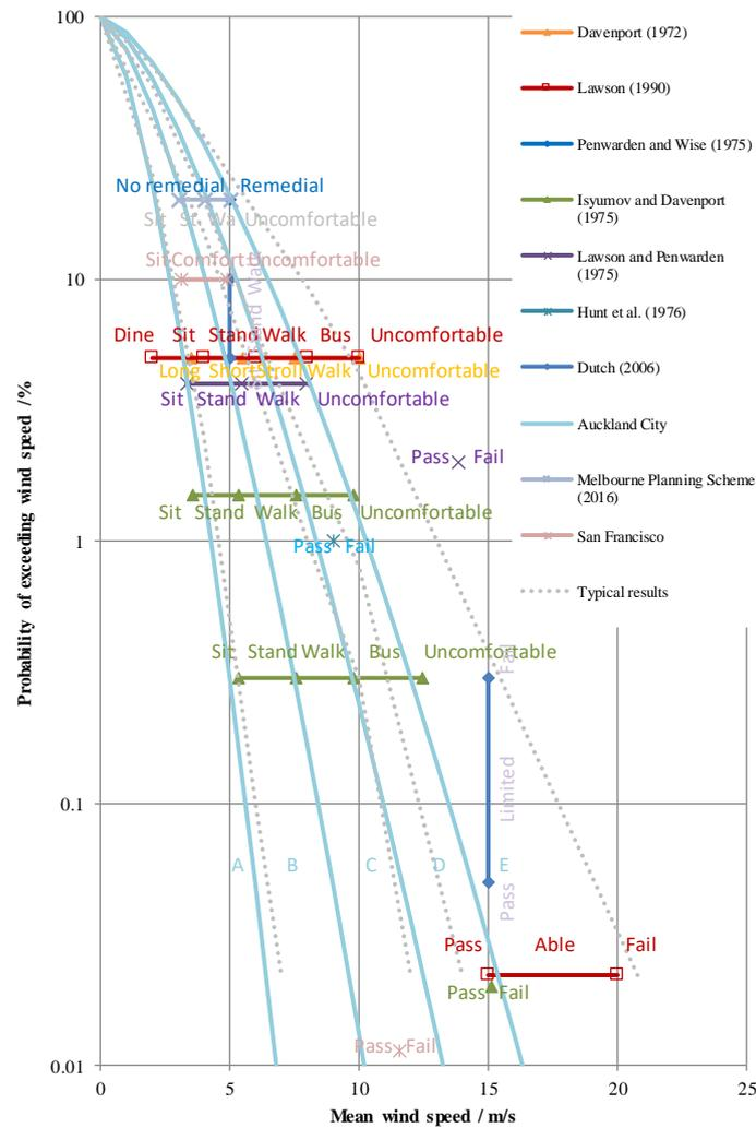
Figure 33 Probabilistic comparison between wind criteria based on mean wind speed
