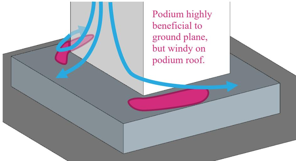
Figure 26 Schematic flow pattern around building with podium
