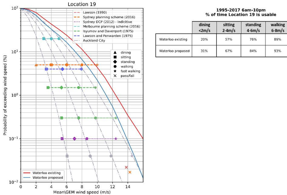
Figure 14: Probabilistic comparison between wind criteria based on mean wind speed (for the hours of 6 am and 10 pm) – Location 19
