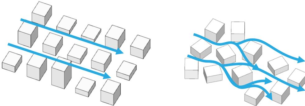
Figure 31 Schematic of flow patterns through a grid and random street layout
